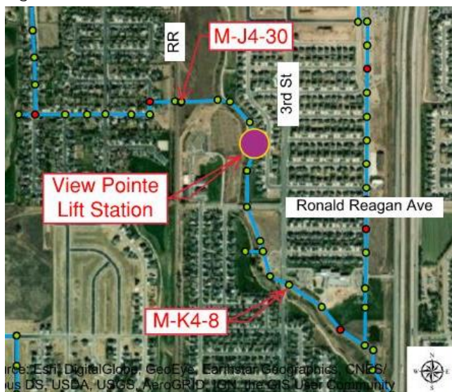
Figure 3-2. Lift Station Elimination Manhole Extents
