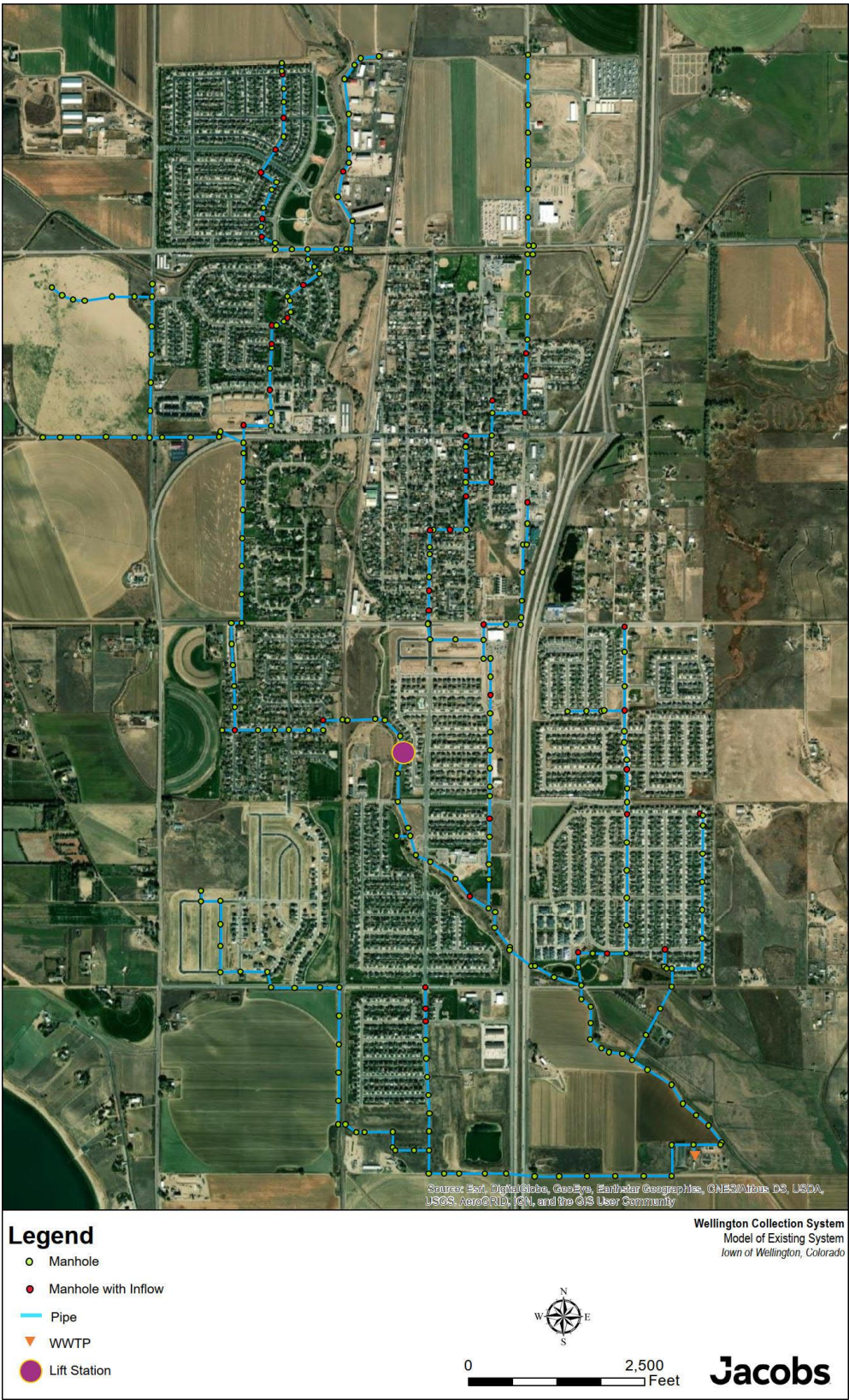
Figure 2-1. Model of Existing Collection System
